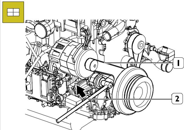
Use specific equipment (2) to install belt (1) on belt tensioner, in direction shown by arrow.
