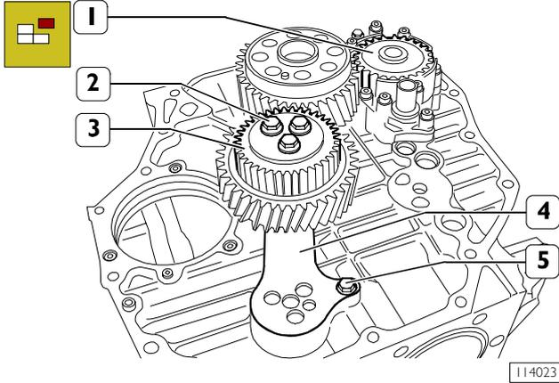
Remove screws (2) and double gear (3).
