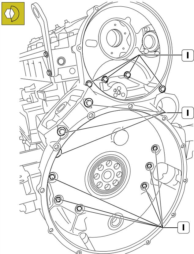
Use torque wrench to lock screws (1) at required torque.
