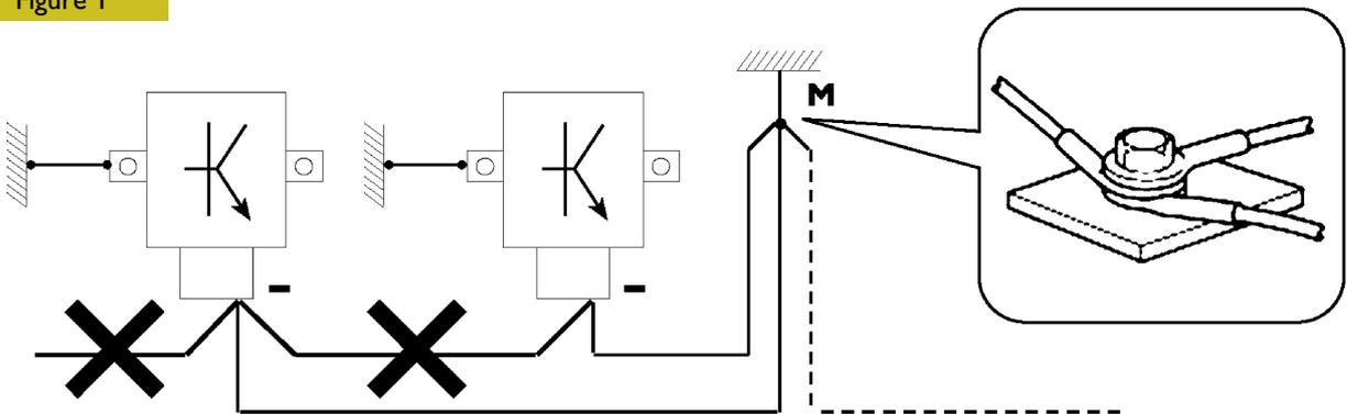
1. NEGATIVE CABLES “STAR” CONNECTION TO SYSTEM BONDING M
