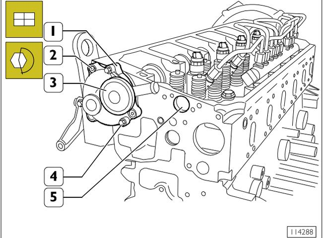
Install blow-by body (1) with related seal and lock screws (2) at required torque.
