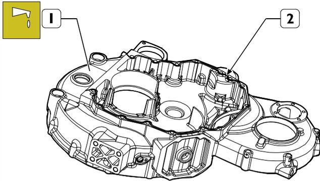
Clean surfaces to be coupled to remove dirt and oil residuals. Apply LOCTITE 275 silicone on gear casing (1) as shown in the figure.
