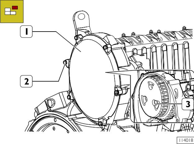
Unlock screws (1) and remove cover (2). Remove centrifugal filter (3) below.
