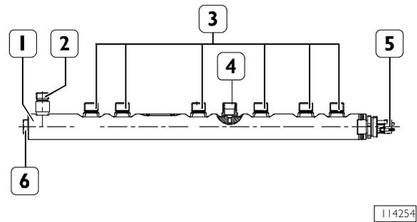
1. Rail - 2. Fuel return - 3. Pipelines to injectors - 4. Fuel supply to high pressure pump - 5. Pressure sensor - 6. Overpressure valve
