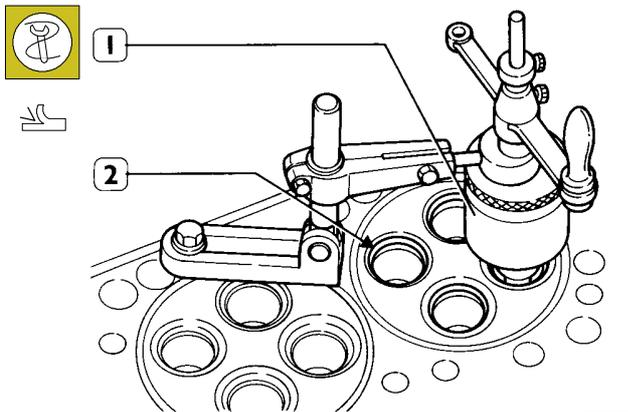
Ream the valve seats (2) on cylinder head using tool (1).
