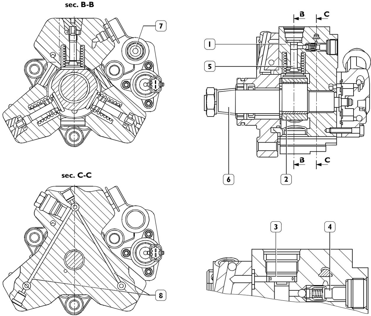
1. Cylinder – 2. Three-lobe element – 3. Cap intake valve – 4. Ball delivery valve – 5. Piston – 6. Pump shaft – 7. Low-pressure fuel inlet – 8. Pumping elements supplying fuel ducts
