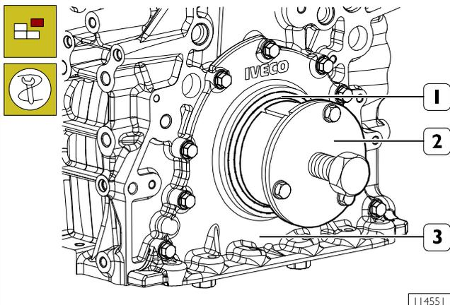
Apply extractor 99340051 (2) and remove seal (1).
