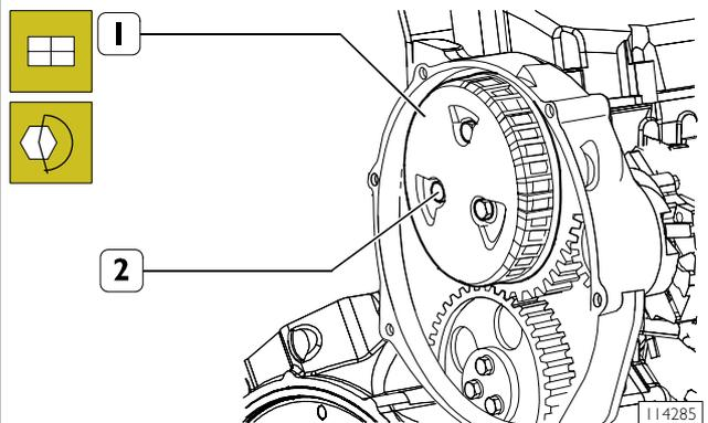
Install centrifugal filter (1) on tune wheel and lock screws (2) at required torque.
