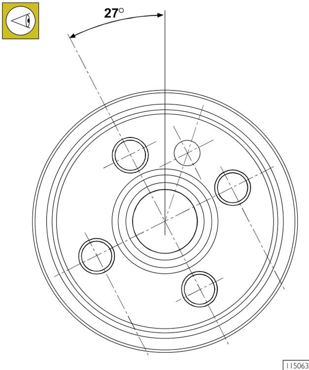
Rotate camshaft by 27° in anticlockwise direction as shown in the figure.
