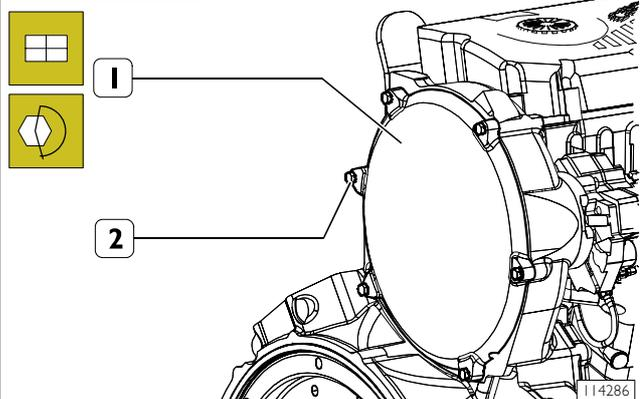
Install timing cover (1) and lock retaining screws (2) at required torque.
