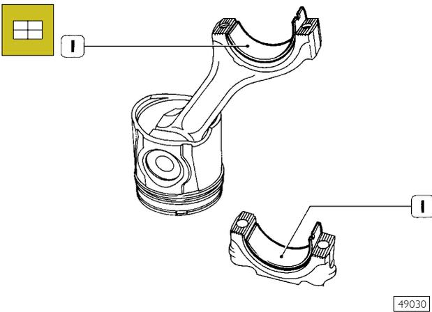
Fit the half-bearings (1), selected as described on pages 19 to 24, both on the connecting rod and on the stand.
