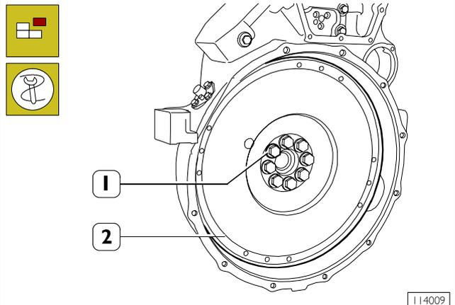
Use specific tool lock engine flywheel (2) rotation, unlock retaining screws (1) and remove engine flywheel.
