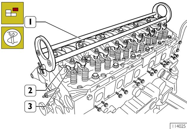
Apply tool 99360558 (1) to rocker arm shaft and remove shaft, remove crosspieces (3) from cylinder head.
