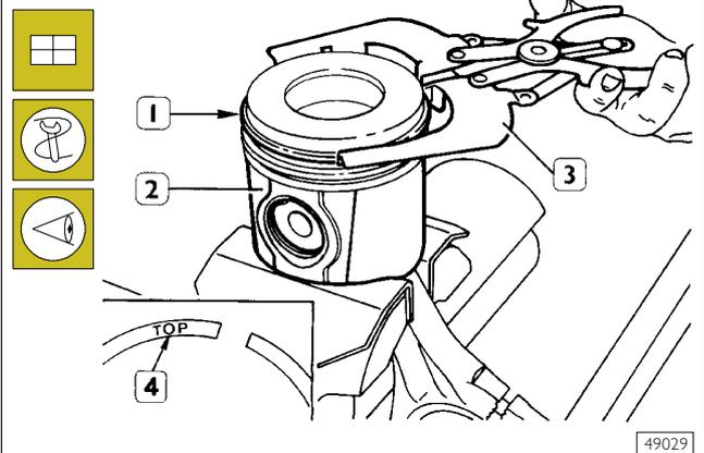
To fit the piston rings (1) on the piston (2) use the pliers 99360184 (3).
