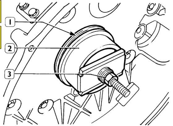
Secure seal (1), install special tool 99346260 (2), lock nut (3) to secure seal.
