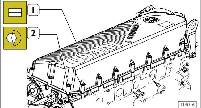
Install cylinder head cover (1) and lock screws (2) at required torque following order shown in Figure 62 diagram.
