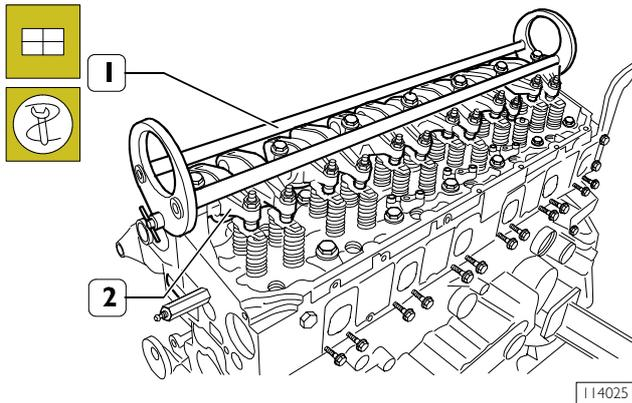
Apply tool 99360558 (1) to rocker arm shaft (2) and install shaft on cylinder head.
