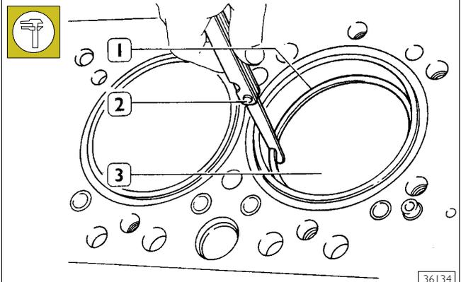
Check the opening between the ends of the sealing rings (1), using a thickness gauge (2), entered in the cylinder barrel (3).
