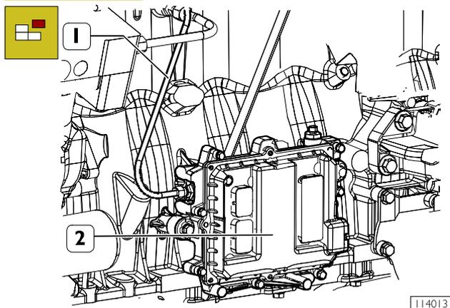
Disconnect line (1) from high pressure pump support and remove ECU (2) with support below.
