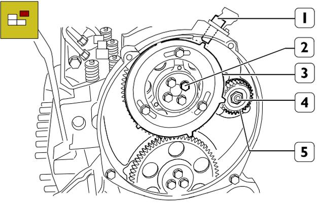
Use specific spanner to unlock screws (2) and remove gear (3) complete with tune wheel.
