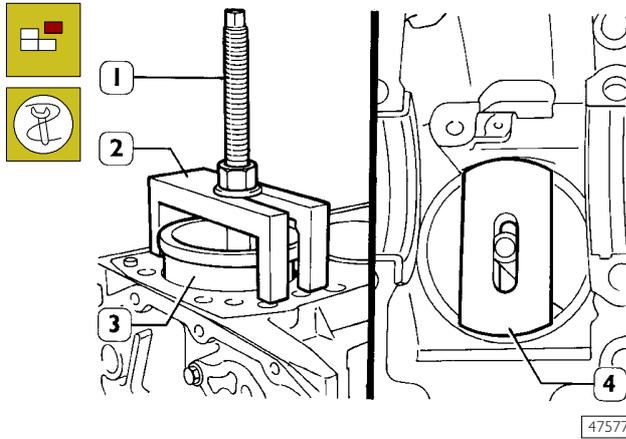
Place details 99360706 (1 and 2) and plate 99360724 (4) as shown in the figure, by making sure that the plate (4) is properly placed on the cylinder liners.
