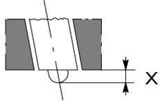
Injector protrusion X                                                                                                               |    | 1.2 to 1.5       |        |
