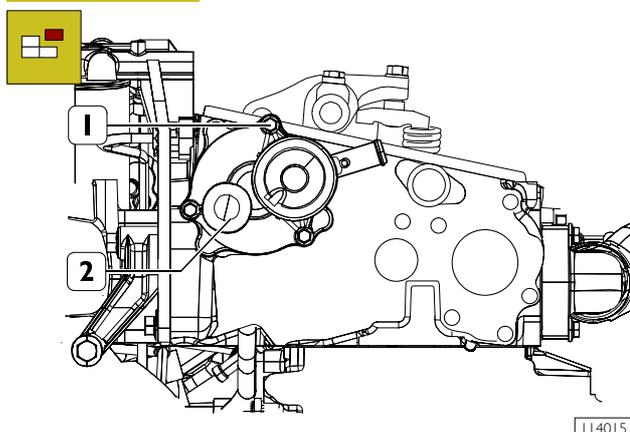
Remove screws (1) and blow-by box (2).
