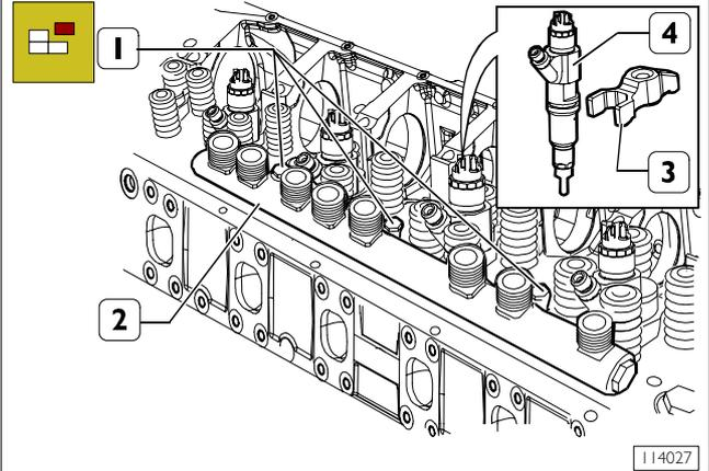
Remove retaining brackets (3) and remove injectors (4).
