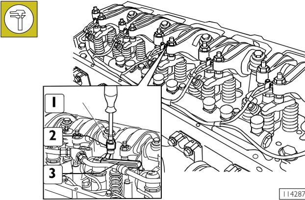
Adjustment of clearance between rocker arms and intake/exhaust valve control crosspieces must be performed with utmost care. Bring to blast phase cylinder to be adjusted; the valves of this cylinder are closed while the symmetric cylinder valves are balanced. Symmetric cylinders are 1-6; 2-5 and 3-4.
