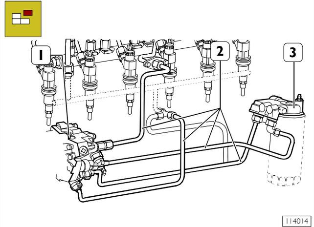
Disconnect fuel lines (2), unlock retaining screws and remove high pressure pump (1). Remove fuel filter support (3) complete with pipeline.
