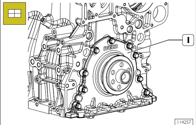
Install front cover (1) and lock retaining screw at required torque.
