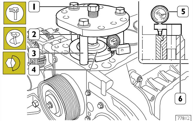
Check cylinder barrel protrusion with tool 99360334 (1-2-3-4) and tighten screw (1) to 170 Nm.
