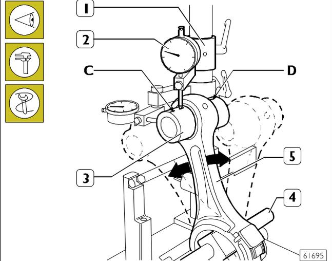
Check the bending of the connecting rod (5) by comparing two points C and D of the pin (3) on the vertical plane of the axis of the connecting rod.
