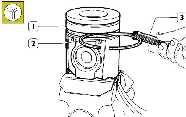
Check the clearance between the sealing rings (2) and the relative piston housings (1) using a thickness gauge (3).
