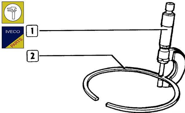
Check the thickness of the piston ring (2) using a micrometer (1).
