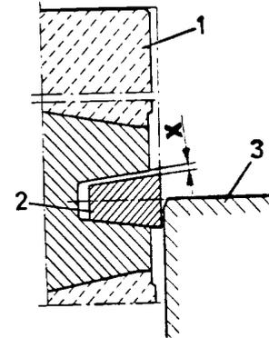
The sealing ring (2) of the 1° cavity is trapezoidal. Clearance "X" between the sealing ring and its housing is measured by placing the piston (1) with its ring in the cylinder barrel (3), so that the sealing ring is half-projected out of the cylinder barrel.
