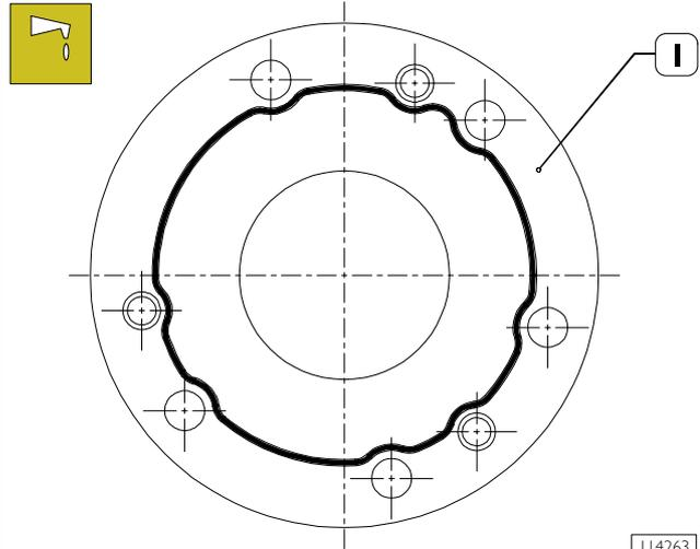
Clean surfaces to be coupled to remove dirt and oil residuals. Apply LOCTITE 275 silicone on gear casing (1) as shown in the figure.
