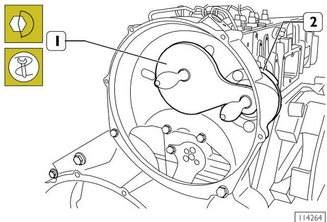
Apply gage 99395221 (1) to check and adjust position of high-pressure pump connection flange (2).
