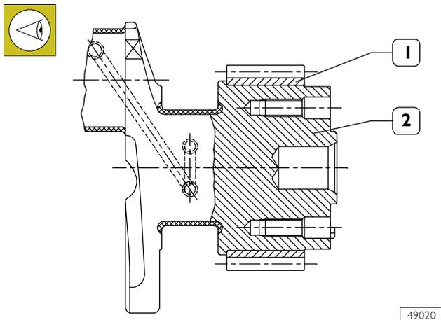
**NOTE** Before fitting the gear, spread Loctite type 603 on approx. 5 mm wide band on crankshaft, at 30 mm from contact surface.
