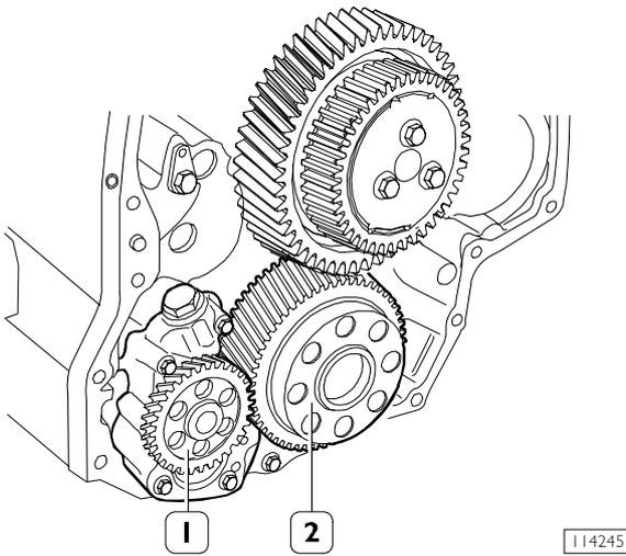
The oil pump (1) cannot be overhauled. On finding any damage, replace the oil pump assembly.
