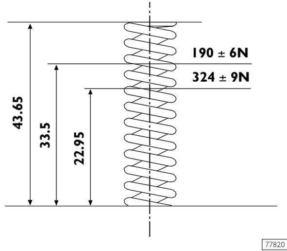
MAIN DATA TO CHECK THE OVERPRESSURE VALVE SPRING
