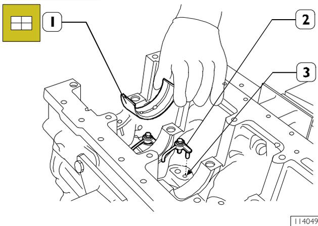
Install the oil spray nozzles (2) and have the dowel coincide with the block hole (3).
