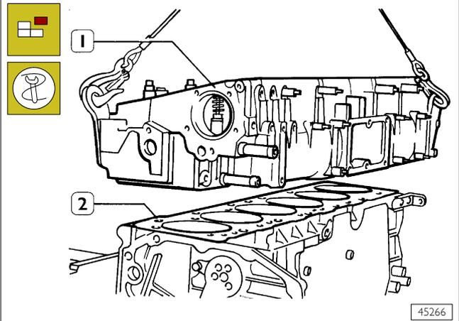
Remove camshaft and remove cylinder head retaining screws.
