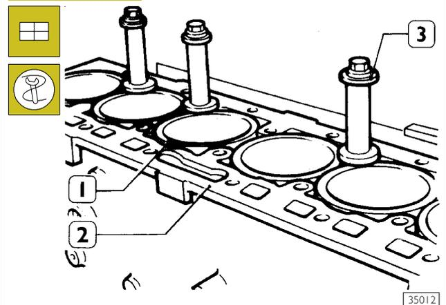
When the installation is completed, block the cylinder liners (1) to the block (2) with studs 99360703 (3).
