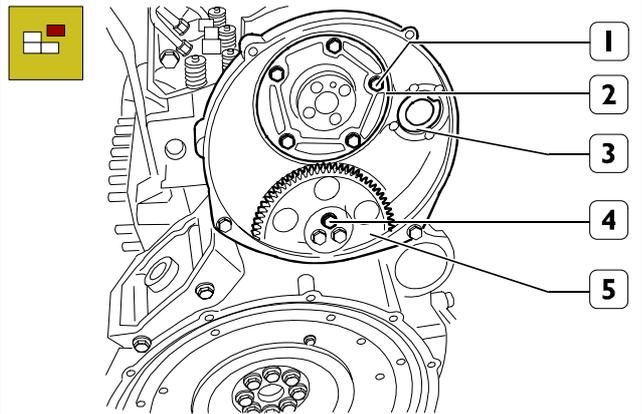
Unlock screws (1) and remove thrust plate (2).
