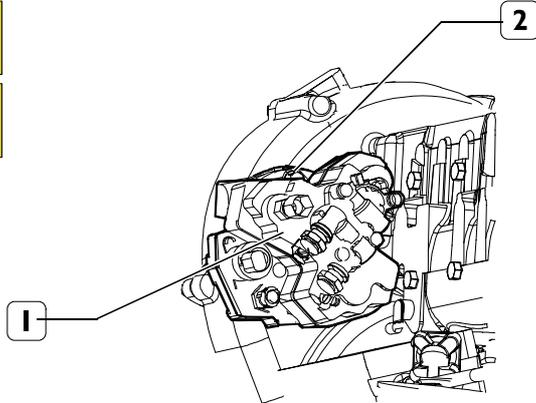
Install high-pressure pump (1) on flange (2).
