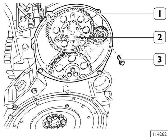
Install gear (1) controlling camshaft so that fastening holes on shaft coincide with slots (2) on control gear.
