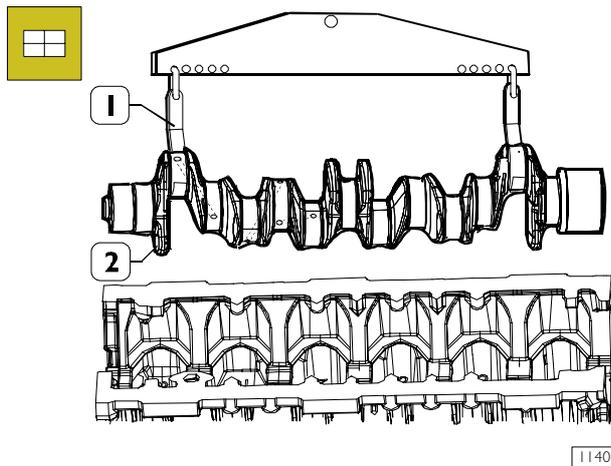
Using the hoist and hook 99360500 (1) mount the driving shaft (2).
