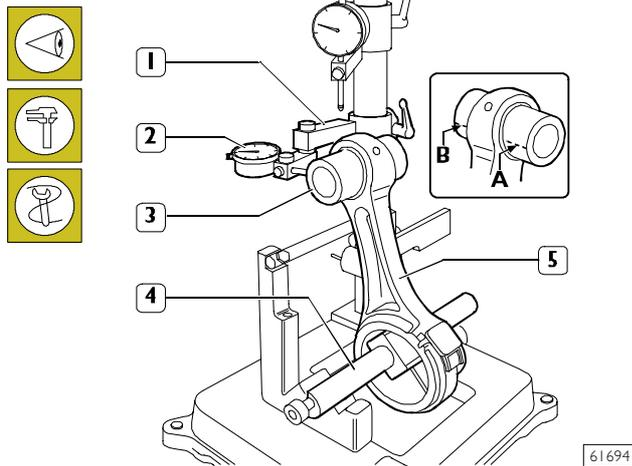
Check the torsion of the connecting rod (5) by comparing two points (A and B) of the pin (3) on the horizontal plane of the axis of the connecting rod.
