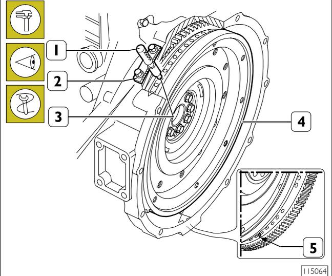
Camshaft is timed if conditions below are found at cam lift values  $4.70 \pm 0.05$ :
