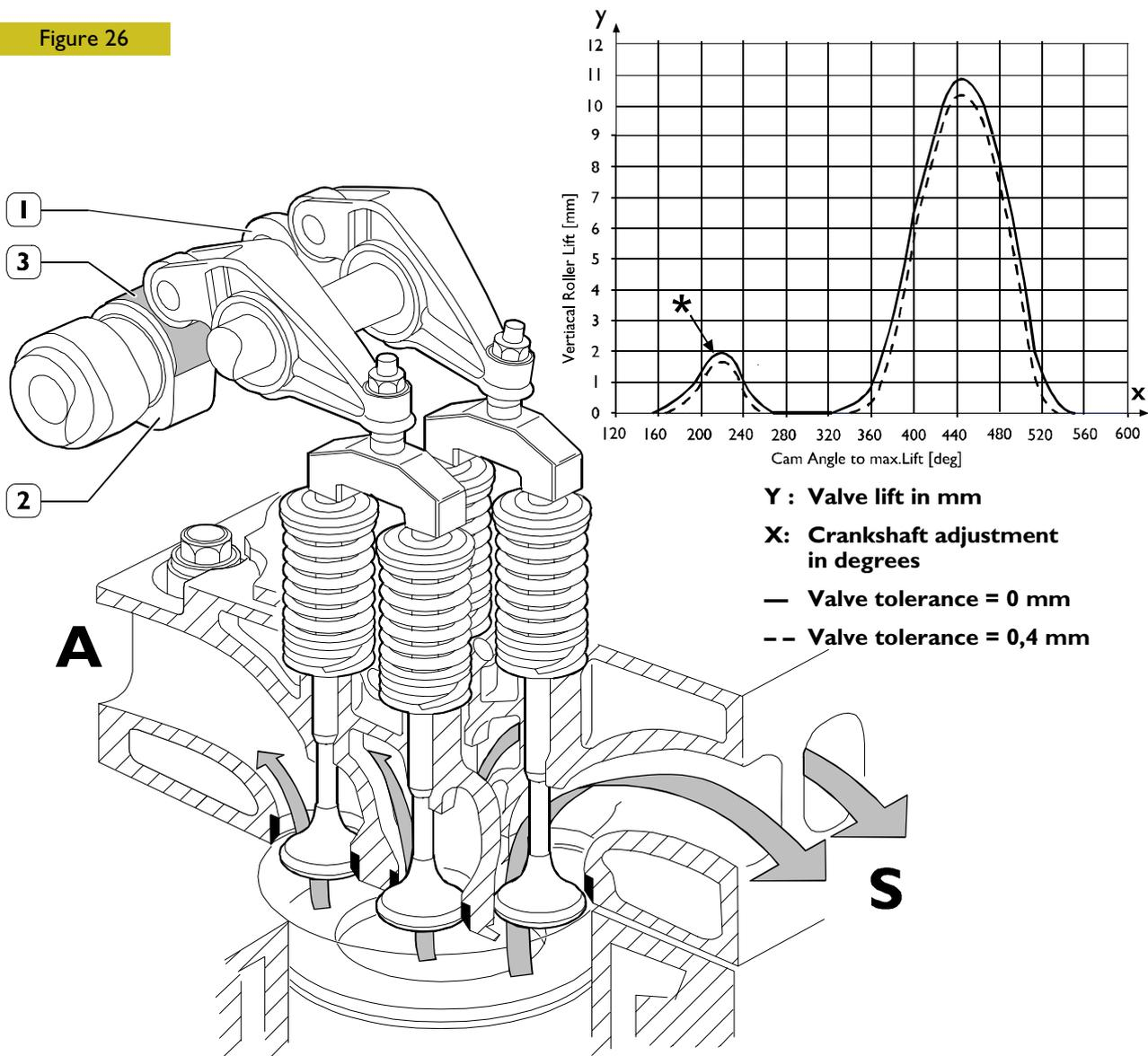
1. Exhaust cams - 2. Suction cams - 3. EGR lobe - S. Exhaust ducts - A. Intake ducts
