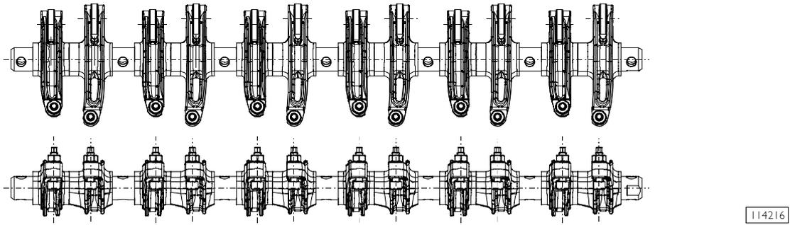
The camshaft eccentric elements control the 12 valve rocker arms directly. Valve control rocker arms are fitted directly on rocker arm shaft. Rocker arms slide directly on cam profiles by rollers. The other end operates on a crosspiece laid directly on the two valve rods. A pad is placed between rocker arm adjustment screw and crosspiece. Two lube ducts are machined inside rocker arms. Rocker arms shaft runs through the cylinder head; it must be removed to reach all units below.
