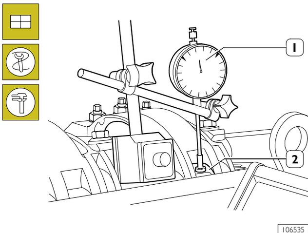
Place dial gage on magnetic base (1) with rod placed on roller (2) of rocker arm controlling cylinder no.3 exhaust valve and apply 6 mm preload.
