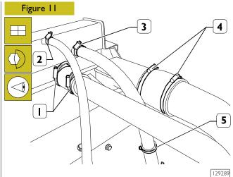
Connect the air and water pipes to the radiator assembly using the clamps (1, 2, 3 and 4) and the mounting bracket (5).
