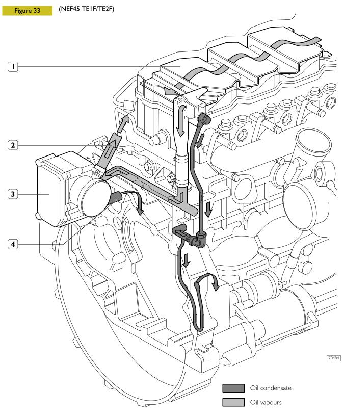
I. Pre-separator - 2. Discharge to the outside (provisional) - 3. Filter - 4. Return to the engine.
