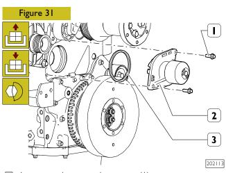
$\hfill \Box$  Loosen and remove the screws (1).
