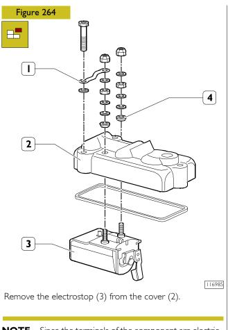
**NOTE** Since the terminals of the component are electrically insulated from the cover, keep in mind the order of assembly of the nuts, washers and the components for the electrical connection of the electrostop terminals; one end is grounded through an appropriate element (1).
