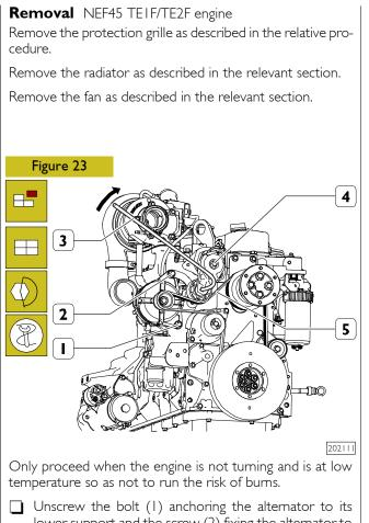
lower support and the screw (2) fixing the alternator to the bracket.
