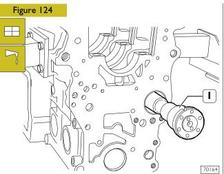
Lubricate the camshaft support bushing and fit the camshaft (1) taking care not to damage the shaft support seats or bushing during this operation.
