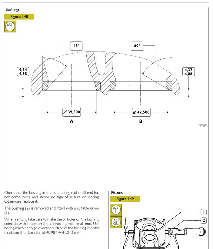
Using a micrometer (2), measure the piston diameter (1) to determine the assembly clearance; The diameter has to be detected at the value indicated in figure.
