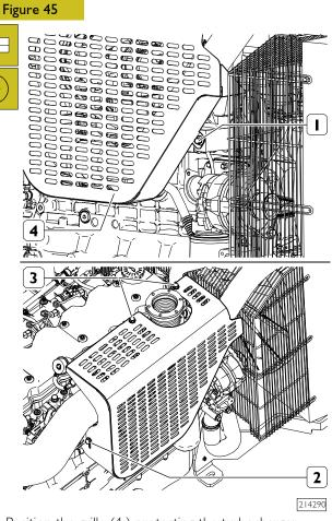
Position the grille (4 ) protecting the turbocharger.
