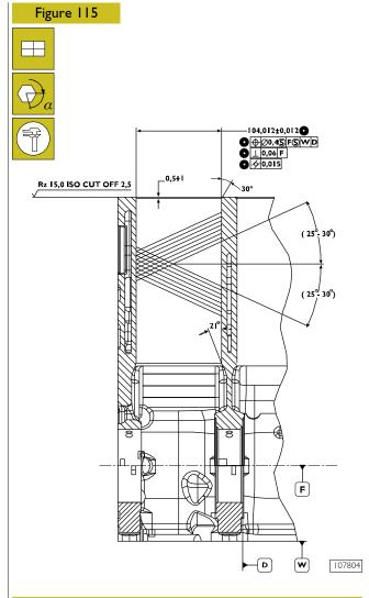
**NOTE** In case of regrinding, all cylinders are to have the same oversize (0.4 - 0.8 mm).
