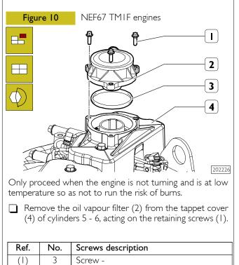
Replace the oil vapour filter (2) and its gasket (3).
