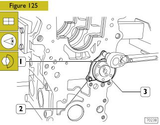
Place the plate (1) retaining the camshaft (3) with the slot facing the top side of the crankcase and the marking facing you, tighten the screws (2).
