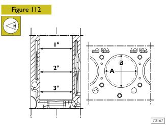
Measurements shall be performed on each cylinder, at three different heights in the bore and on two planes perpendicular with each other: one parallel to the longitudinal axis of the engine (A) and the other perpendicular to it (B); the greatest wear is usually found to be on this surface and during the first measurement.
