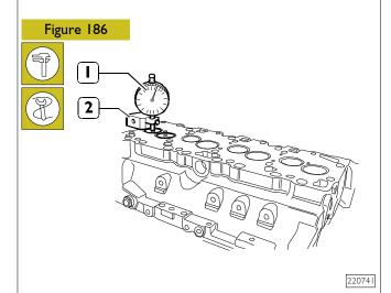
After regrinding, check that valve (3) recessing value is the specified one by using the stand 99370415 (2) and the dial gauge 99395603 (1).
