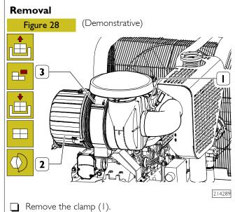
Unscrew the screws (3) and remove the air filter (2) from its support.
