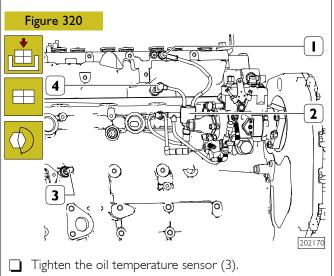
Tighten the water temperature sensor (4).
