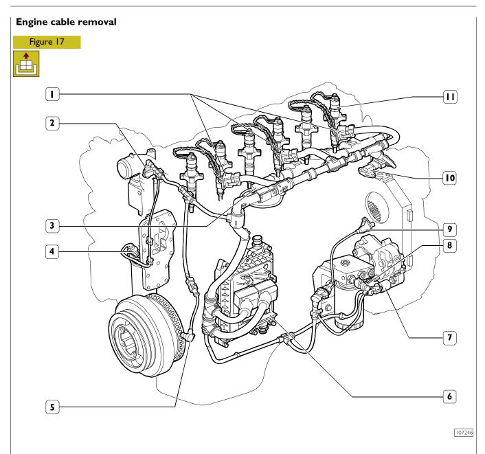
I. Connections for electro-injectors - 2. Engine coolant temperature sensor - 3. Fuel pressure sensor cable - 4. Engine oil temperature and pressure sensor - 5. Crankshaft sensor - 6. EDC control unit 7 - 7. Pressure regulator cable - 8. Fuel heater and fuel temperature sensor cable - 9. Timing phase sensor - 10. Air temperature and pressure sensor - 11. Electro-injector.
