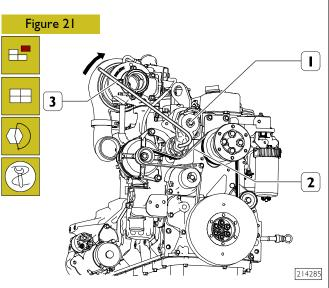
Using tool (3), loosen the automatic belt tensioner (1).Remove the belt (3).
