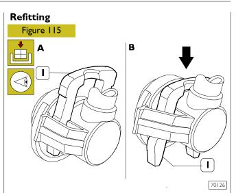
To connect lower pressure fuel pipes from their couplings, press clip (1) as shown in figure B.
