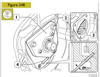
Apply the tool 99360339 (1) to the flywheel housing to stop the rotation of the flywheel (3), using an adjustable wrench on the nut (2) and a pin (4).
