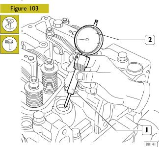
To search for the position of 1<sup>st</sup> cylinder at top dead, end of compression stroke, remove the rocker arm cover of the 1<sup>st</sup> cylinder, remove the 1<sup>st</sup> injector and position the tool (1). pre-load the dial gauge.
