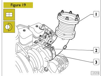
Connect the discharge pipe (1), tightening the screw (2) to close the clamp (3).
