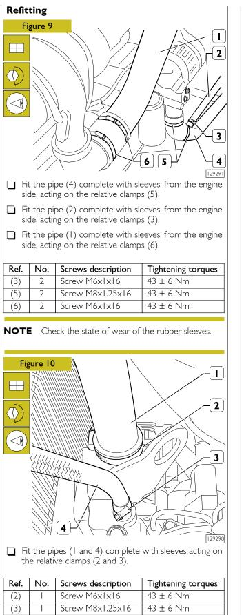
**NOTE** Check the state of wear of the rubber sleeves.
