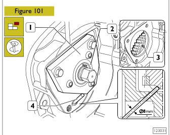
Once the starter motor is removed, fit tool 99360339 (1) to rotate the flywheel.
