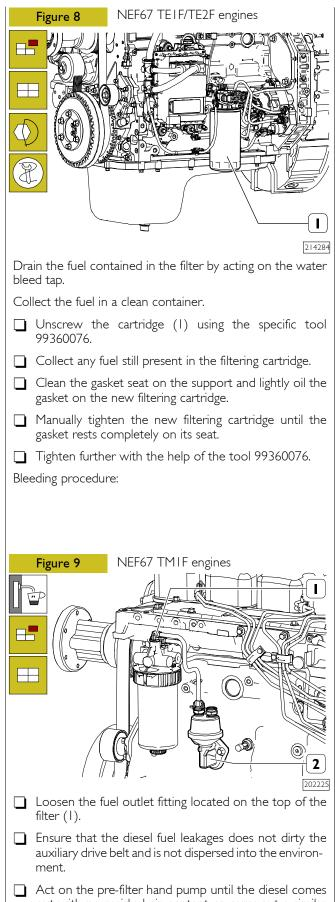
Start the engine and run it at idle for a few minutes to remove any residual air.
