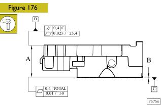
The rated thickness A for the cylinder head is  $95 \pm 0.25$  mm, max. metal removal must not exceed thickness B by 0.13 mm.
