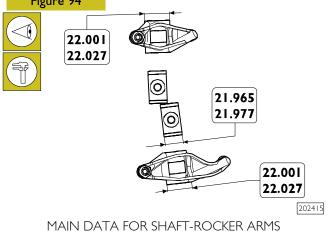
Check the coupling surfaces between the support and the shaft: there must be no sign of excessive wear or damage. Replace if necessary.
