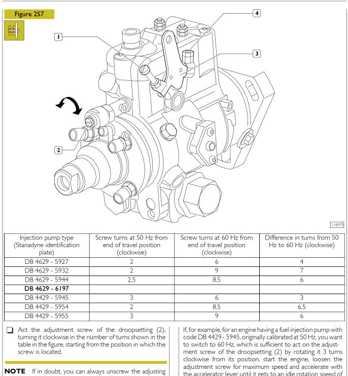
screw of the droopsetting (2) counter-clockwise until you reach the end - do not force further, to prevent damage to the control system.
