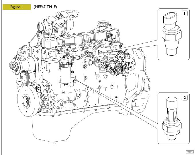
I. Water temperature sensor - 2. Oil pressure sensor
