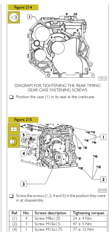
**NOTE** Before each assembly operation, check that the thread on the holes and the screws shows no sign of wear or dirt.
