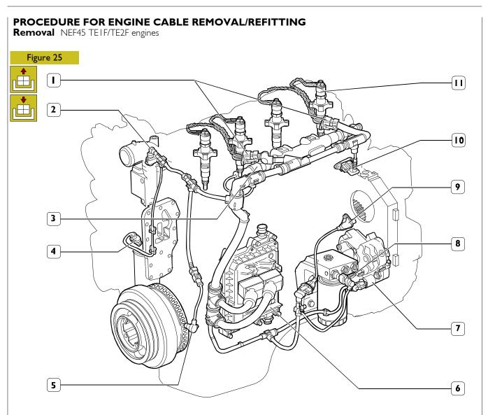
I. Connections for electro-injectors - 2. Engine coolant temperature sensor - 3. Fuel pressure sensor cable - 4. Engine oil temperature and pressure sensor - 5. Crankshaft sensor - 6. EDC control unit 7 - 7. Pressure regulator cable - 8. Fuel heater and fuel temperature sensor cable - 9. Timing phase sensor - 10. Air temperature and pressure sensor - 11. Electro-injector.
