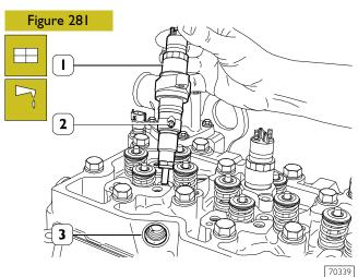
Fit injectors (1) on the cylinder head seats, directed so that the fuel inlet hole (2) is facing the fuel manifold seat (3) side.
