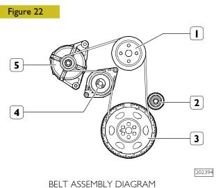
BELT ASSEMBLY DIAGRAM I. Fan pulley - 2. Idler pulley - 3. Crankshaft pulley -4. Water pump - 5. Alternator
