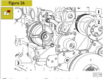
Unscrew the screw (3) anchoring the alternator to its lower support and the screw (1) securing it to the bracket (2).
