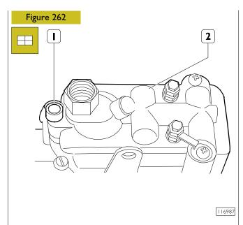
The placement of the cover (2) should be carried out in the reverse order to what is described about the disassembly, taking care that it fits perfectly on the mounting seat, without forcing (obviously for the ETR variant the pump cover will fit on the mounting seat only after the removal of the retaining tool).
