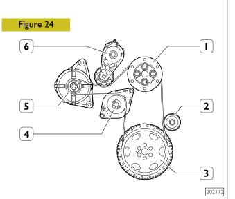
BELT ASSEMBLY DIAGRAM I. Fan pulley - 2. Idler pulley - 3. Crankshaft pulley -4. Water pump - 5. Alternator -6. Automatic belt tensioner
