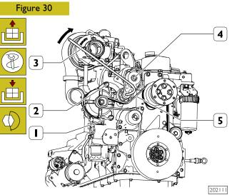
Unscrew the screw (1) anchoring the alternator to its lower support and the screw (2) securing the bracket.
