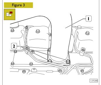
Unscrew the screws (2) and remove the pipe (1) from the intake manifold.
