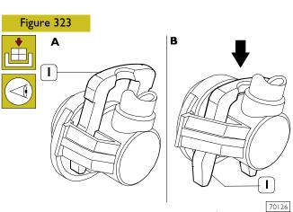
To connect lower pressure fuel pipes from their couplings, press clip (1) as shown in figure B.
