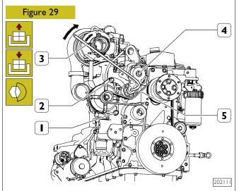
Unscrew the screws (2 and 4) anchoring the alternator (5) to its support and the screw (1) adjusting the position of the alternator.
