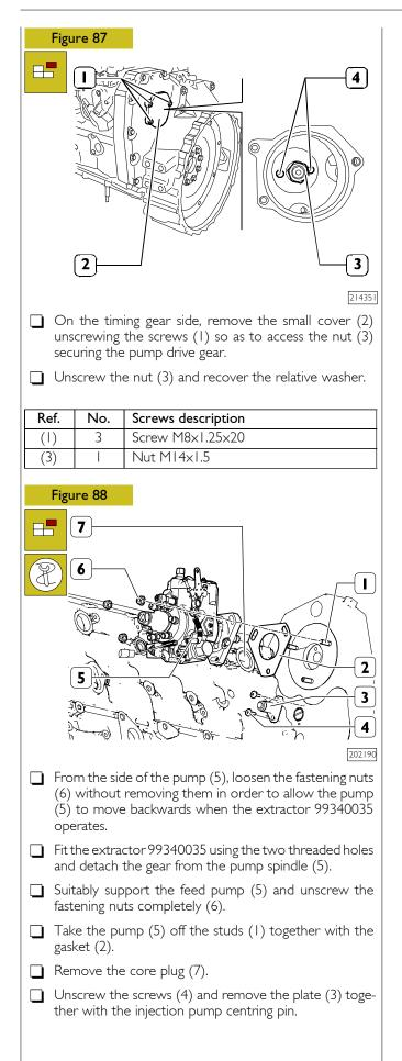
**NOTE** Support the pump drive gear to prevent interference or sticking when the timing gears rotate.
