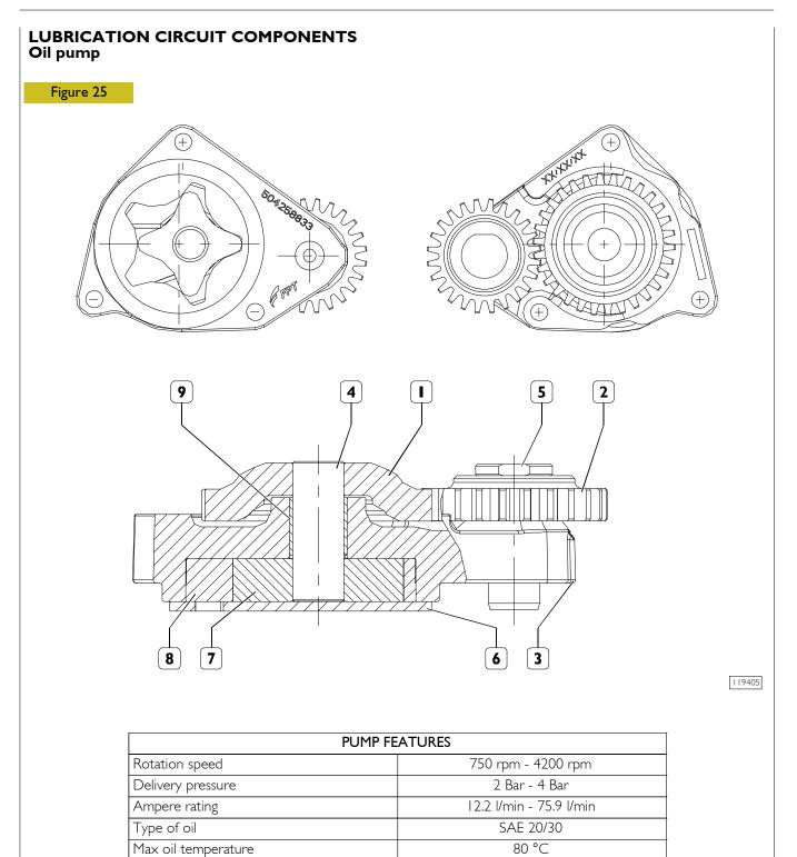
Primary gear - 2. Secondary gear - 3. Pump body - 4. Control shaft - 5. Layshaft
