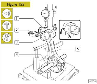
Check the torsion of the connecting rod (5) by comparing two points (**A** and **B**) of the pin (3) on the horizontal plane of the axis of the connecting rod.
