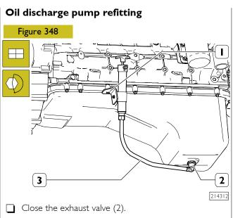
Position the oil discharge pump (3) and tighten the screw (1).
