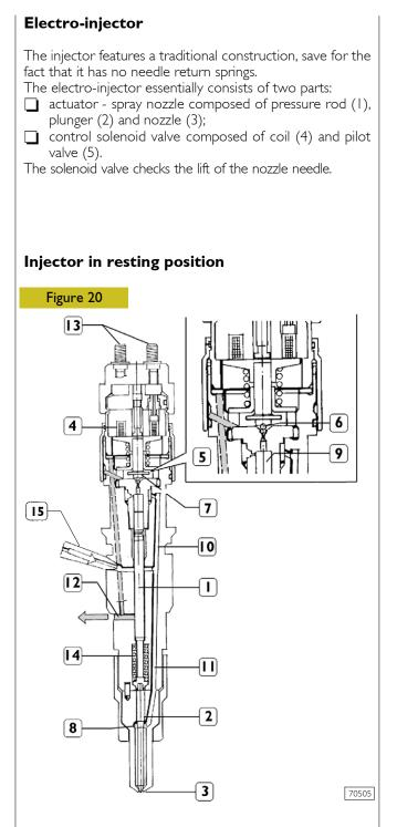
Pressure rod - 2. Needle - 3. Nozzle -4. Coil - 5. Pilot valve - 6. Ball shutter Control area - 8. Pressure chamber - 9. Control volume 10. Control duct - 11. Supply pipe - 12. Control fuel outlet -13. Power connection - 14. Spring -15. High pressure fuel inlet.
