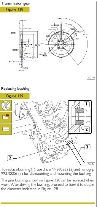
**NOTE** The hammering of the bushing into the gear must be carried out in the direction of the arrow by placing it at the point indicated inFigure 128.
