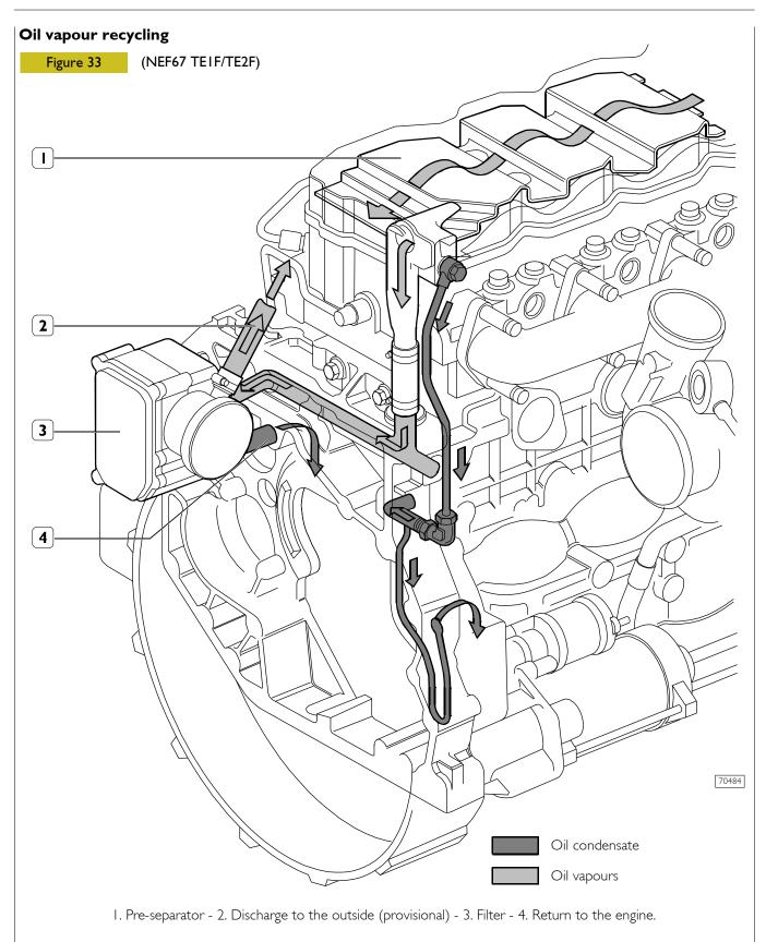
The tappet cover houses the pre-separator (1), whose shape and position determines an increase in oil vapour outlet speed and condenses a part of the vapours at the same time.
