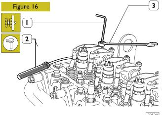
Registration of the clearance between the rocker arms and crossbars which control the intake and exhaust valves must be carried out carefully using the hex key (1) box wrench (3) and feeler gauge (2).
