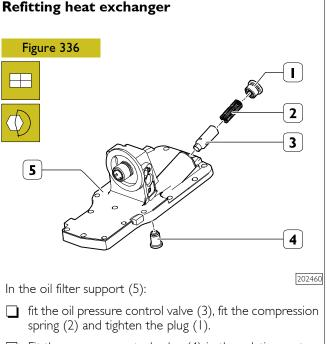
Fit the pressure control valve (4) in the relative seat.
