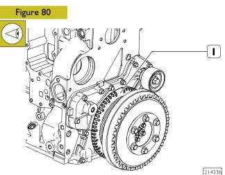
Make sure that the non-drilled part (1) of the phonic wheel is positioned at the top along its vertical axis.
