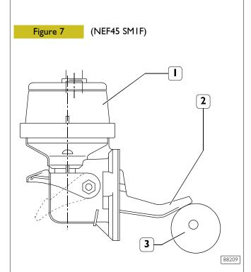
I. Pump - 2. Control lever - 3. Camshaft.
