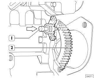
Rotate the flywheel until it pushes the pin 99360616 (1), this will not block the gear (2), obtaining the TDC of the  $1^{st}$  cylinder.
