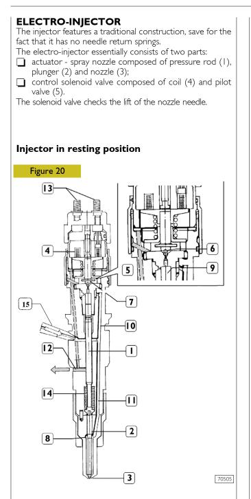
Pressure rod - 2. Needle - 3. Nozzle -4. Coil - 5. Pilot valve - 6. Ball shutter Control area - 8. Pressure chamber - 9. Control volume 10. Control duct - 11. Supply pipe - 12. Control fuel outlet -13. Power connection - 14. Spring -15. High pressure fuel inlet.
