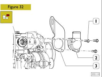
Unscrew the screws (1) securing the thermostat cover (2).
