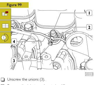
Remove the injector exhaust pipe (4).
