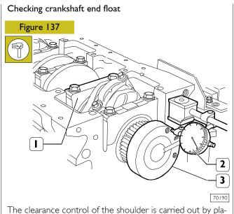
The clearance control of the shoulder is carried out by placing a dial gauge (2) to the magnetic base on the crankshaft (3) as shown in the figure, the normal mounting clearance is  $0.068 \div 0.410$  mm.
