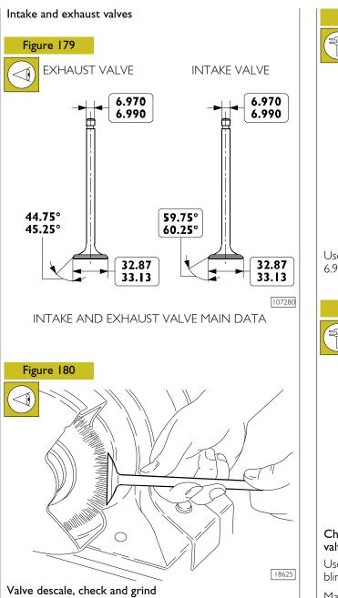
Remove all carbon deposits from the valves using a wire brush. Check that the valves show no signs of seizing, cracks or burns.
