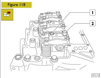
Disassemble the rocker arm mounts:
