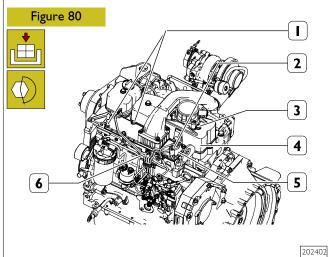
Tighten the screws (6) securing the support plate.
