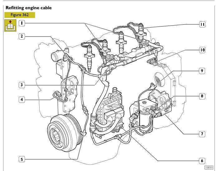
I. Connections for electro-injectors - 2. Engine coolant temperature sensor - 3. Fuel pressure sensor cable - 4. Engine oil temperature and pressure sensor - 5. Crankshaft sensor - 6. EDC control unit 7 - 7. Pressure regulator cable - 8. Fuel heater and fuel temperature sensor cable - 9. Timing phase sensor - 10. Air temperature and pressure sensor - 11. Electro-injector.
