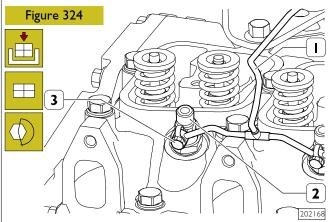
Position the exhaust pipes (1) from the injectors (2).
