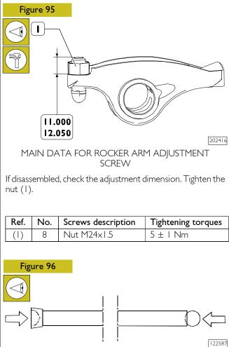
Before assembly, check the rocker arm rods: there must be no sign of any deformation; the spherical seats for contact with the rocker arm adjusting screw and with the tappets (arrows) must show no trace of seizure or wear; if they do, replace them.
