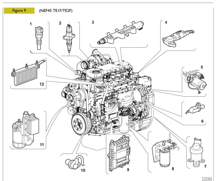
The NEF F4HE engines are entirely managed by the electronic control unit. This is mounted directly on the engine by means of a heat exchanger that allows the cooling, using the elastic plugs which reduce the vibrations transmitted from the engine.
