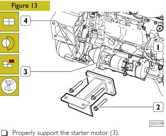
Loosen the retaining nuts (1).
