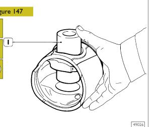
Lubricate the pin (1) and the relevant housing on the piston hubs with engine oil; Pin must be inserted in the piston with a light finger pressure and it should not come out by gravity.
