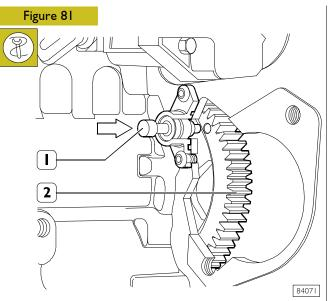
Rotate the flywheel until it pushes the pin 99360616 (1), this will not block the gear (2), obtaining the TDC of the  $1^{st}$  cylinder.
