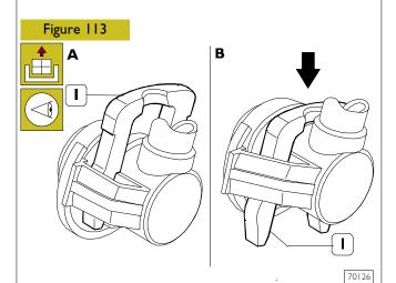
To disconnect lower pressure fuel pipes from their couplings, press clip (1) as shown in figure B.
