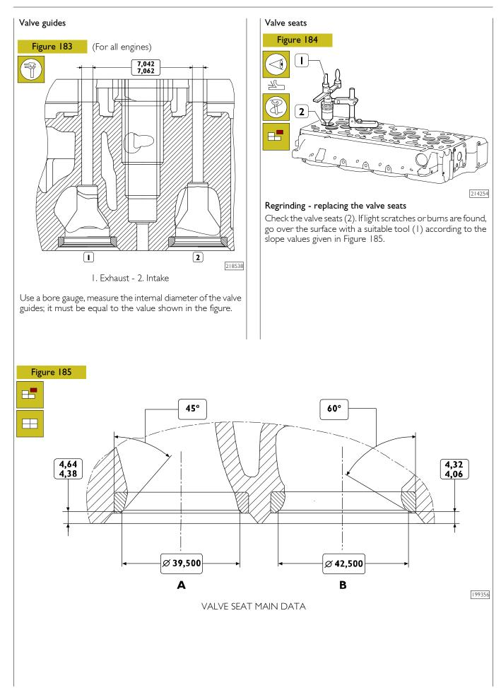
If valve seats cannot be restored just by regrinding, it is possible to replace them with spare seats.
