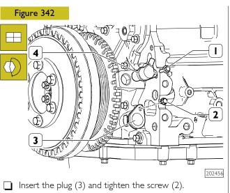
Insert the crankshaft rpm sensor (4) and tighten the screw (1).
