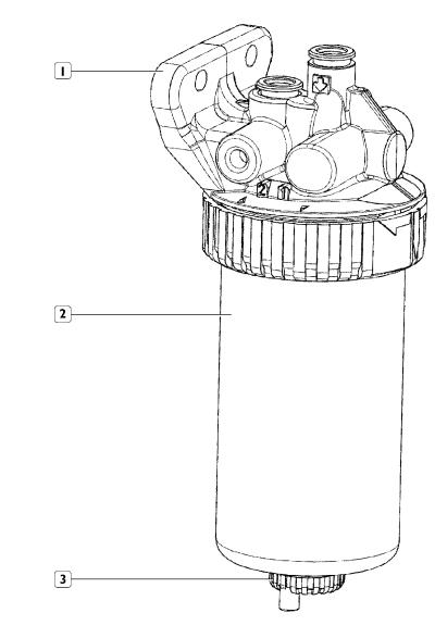
I. Fuel filter support - 2. Filtering cartridge - 3. Water bleed screw.
