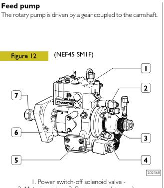
Metering valve - 3. Pressure regulator unit Hydraulic head - 5. Automatic advance - 6. Seat 7. Propeller shaft
