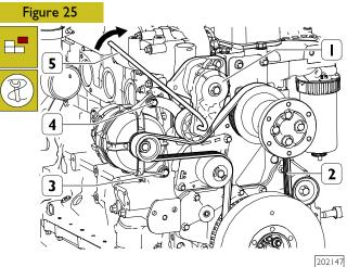
Loosen the screw (3) anchoring the alternator to its lower support and the bolt (4) fixing the alternator to the bracket.
