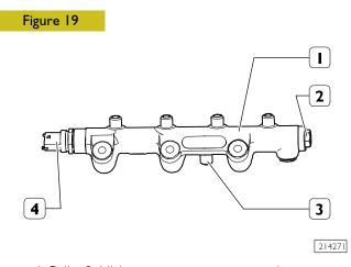
Rail. - 2. High pressure overpressure valve. -3 Entrance of fuel from the pump -4. Pressure sensor.
