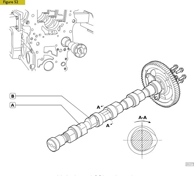
A. Intake valve control - B. Exhaust valve control.
