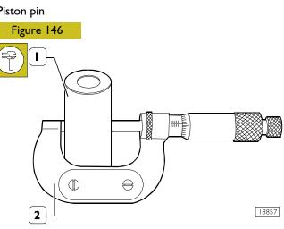
Measuring the diameter of the gudgeon pin (1) with a micrometer (2).
