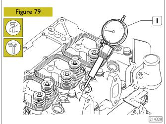
To search for the position of I<sup>st</sup> cylinder at top dead, end of compression stroke, remove the rocker arm cover of the I<sup>st</sup> cylinder, remove the I<sup>st</sup> injector and position the tool (99395097 (1). Pre-load the dial gauge 99395604.
