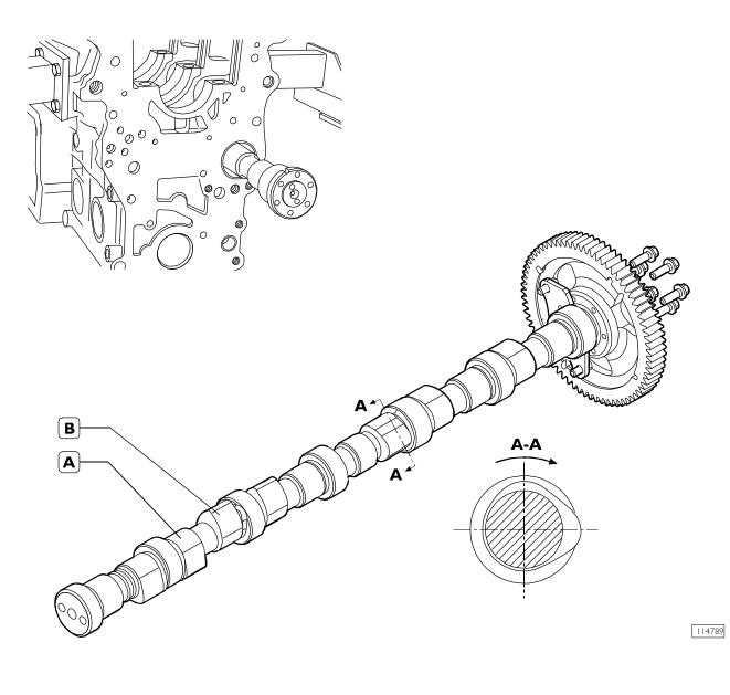
A. Intake valve control - B. Exhaust valve control.
