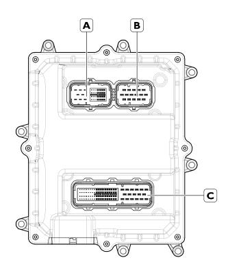
A. Sensor connector - B. Injector connector - C. Chassis side connector
