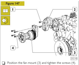
Position the automatic belt tensioner (2) and tighten the screws (1).
