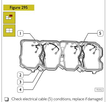
by cutting the support (2) clamps and removing the screws (4) that secure it to the connections (3).
