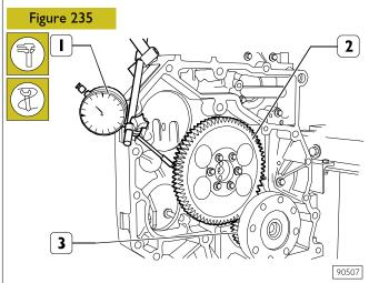
Set the dial gauge 99395604 (1) on the timing gear (2) and check that the clearance between the gears (2) and (3) is between 0.076 and 0.280 mm.
