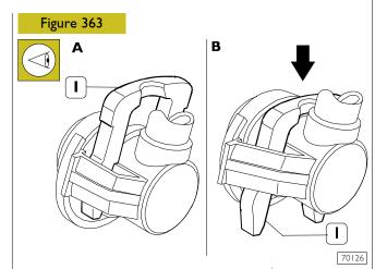
To connect lower pressure fuel pipes from their couplings, press clip (1) as shown in figure B.
