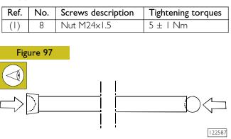
Before assembly, check the rocker arm rods: there must be no sign of any deformation; the spherical seats for contact with the rocker arm adjusting screw and with the tappets (arrows) must show no trace of seizure or wear; if they do, replace them.
