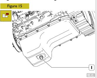
Drain the oil through the plug (1) located below the oil sump.
