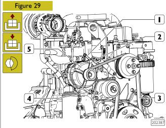
Unscrew the screws (2 and 4) anchoring the alternator (5) to its support and the screw (1) adjusting the position of the alternator.
