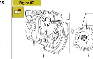
214351 On the timing gear side, remove the small cover (2) unscrewing the screws (1) so as to access the nut (3)
