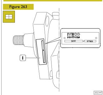
If replacing the electrostop originally supplied and changing the characteristics (different voltage, ETR rather than ETSO, etc.), you must apply a plate (1) identifying the area indicated.
