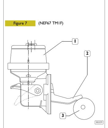
I. Pump - 2. Control lever - 3. Camshaft.
