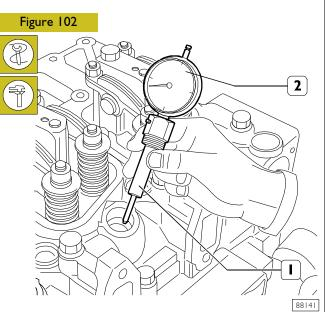
To search for the position of 1<sup>st</sup> cylinder at top dead, end of compression stroke, remove the rocker arm cover of the 1<sup>st</sup> cylinder, remove the 1<sup>st</sup> injector and position the tool (1). pre-load the dial gauge.
