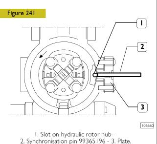
The synchronisation pin 99365196 (2) has been designed for use in the event that the rotor shaft has been accidentally
