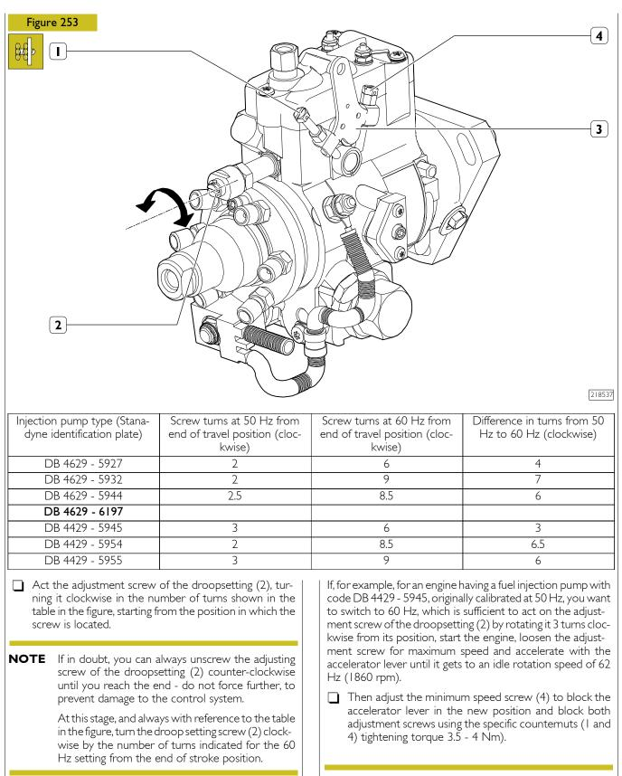
**NOTE** The idling speed adjustment screw (4) does not allow achievement of the minimum in the "classic" sense of the term, as the injection pump regulator imposes a higher rotation speed since it is the injection pump for the generator unit.
