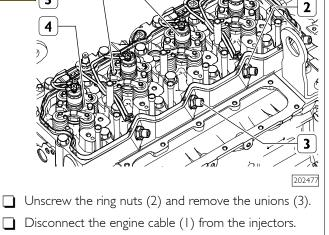
Unscrew the screws (5) and remove the brackets (4) fixing the injectors (6).
