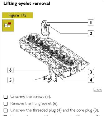
$\Box$  Unscrew the screws (1) and remove the lifting eyelet (2).
