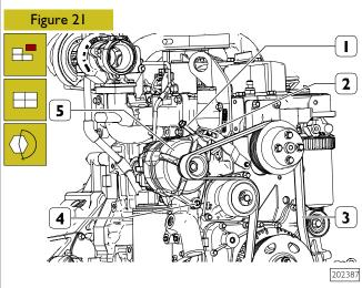
Remove the protective grille and the fan together with spacer by acting on the relative fasteners.
