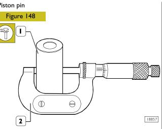
Measuring the diameter of the gudgeon pin (1) with a micrometer (2).
