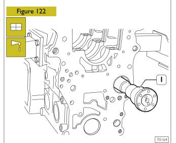
Lubricate the camshaft support bushing and fit the camshaft (1) taking care not to damage the shaft support seats or bushing during this operation.
