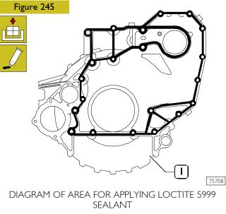
Perfect seal is only obtained by cleaning accurately the surface to seal.
