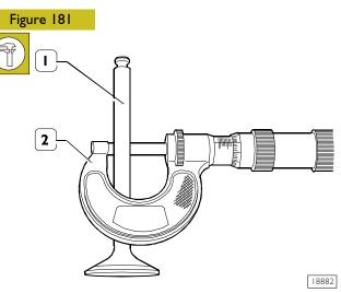
Use micrometer (2) to measure valve (1) stem: it must be 6.990  $\div$  7.01 mm
