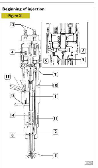
When coil (4) is energised, it makes shutter (6) move upwards. The control volume (9) fuel flows towards flow duct (12) making a pressure drop occur in control volume (9). Simultaneously the fuel pressure into pressure chamber (8) makes plunger (2) lift, with following fuel injection into the cylinder.
