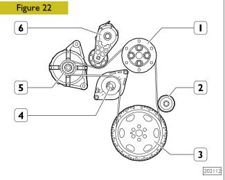
BELT ASSEMBLY DIAGRAM I. Fan pulley - 2. Idler pulley - 3. Crankshaft pulley -4. Water pump - 5. Alternator
