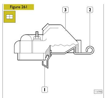
In the electrostop **ETR** kit there is the joint tool (1) which must be used to position the electrostop arm (2) correctly and to reassemble the cover on the injection pump.
