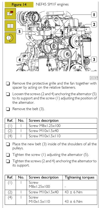
Reposition the fan together with spacer in its seat and the protective grilles and tighten the relative fasteners.
