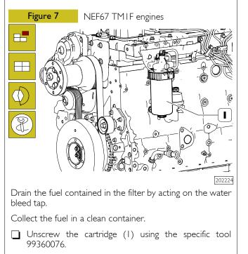
Collect any fuel still present in the filtering cartridge.
