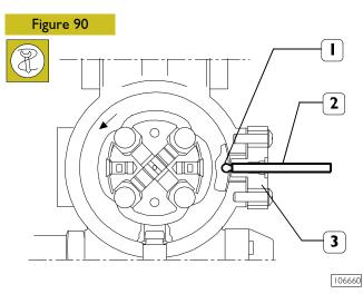
I. Slot on hydraulic rotor hub - 2. Synchronisation pin 99365196 - 3. Plate.
