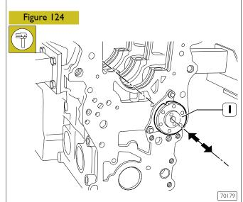
Check the axial clearance of the camshaft (1). It must be  $0.23 \pm 0.13$  mm.
