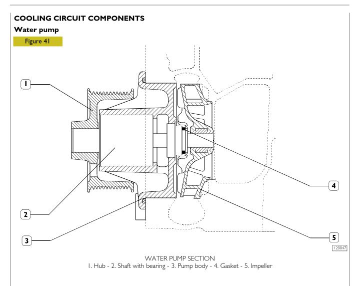
The water pump is of the vane centrifugal type. The pump bearing (2) forms a single piece with the spindle of the impeller. The water seal between the pump body (3) and the spindle (2) is obtained by the gasket (4).
