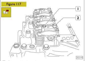
Disassemble the rocker arm mounts:
