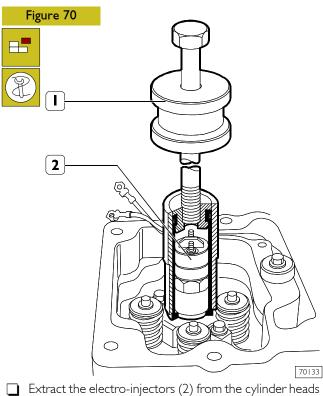
Extract the electro-injectors (2) from the cylinder head with tool 99342101 (1).
