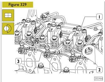
Tighten the fittings (2) connecting to the injectors.
