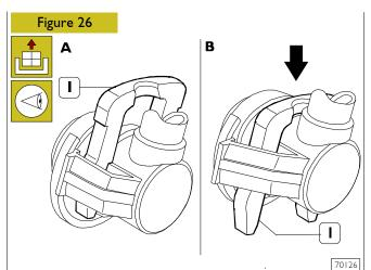
To disconnect lower pressure fuel pipes from their couplings, press clip (1) as shown in figure B.
