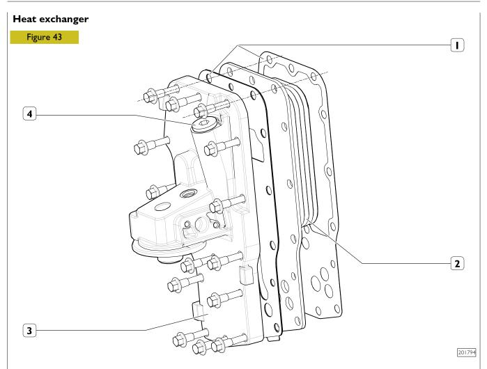
I. Gaskets - 2. Internal heat exchanger element (7 elements) - 3. Heat exchanger body -4. Pressure regulator valve
