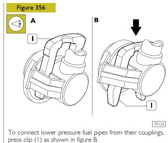
After removing the pipe, move the clip (1) to the locked position (Figure A).
