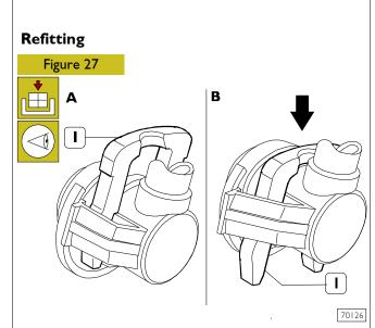
To connect lower pressure fuel pipes from their couplings, press clip (1) as shown in figure B.
