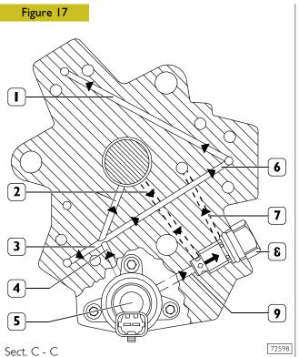
Plunger inlet - 2. Pump lubrication pipes - 3. Plunger inlet - 4. Main plunger supply pipe - 5. Pressure regulator -6. Plunger inlet - 7. Regulator drainpipe - 8. Pressure limiting valve 5 bar - 9. Fuel discharge from regulator inlet.
