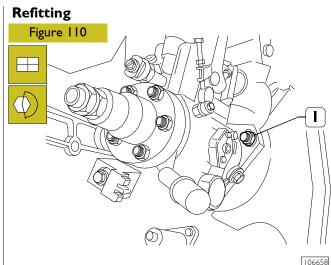
When fitting the feed pump on the engine, the conditions of the T.D.C at the  $I^{st}$  cylinder at the end of the compression stroke must be met.
