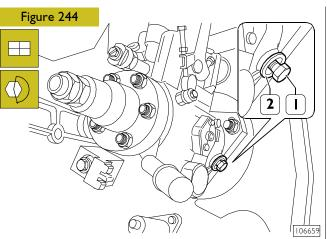
Tighten the screw (1) locking the pump spindle.
