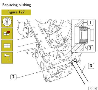
To replace bushing (1), use driver 99360362 (2) and handgrip 99370006 (3) for dismounting and mounting the bushing.
