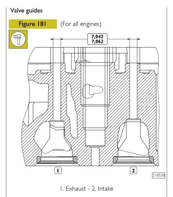
Use a bore gauge, measure the internal diameter of the valve guides; it must be equal to the value shown in the figure.
