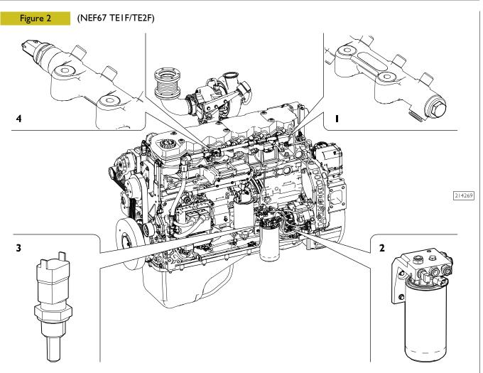
Pressure regulation valve on Rail - 2. Fuel heater on filter -3. Fuel temperature sensor - 4. Pressure sensor on Rail
