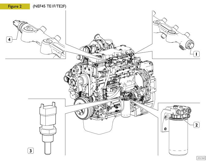
Pressure regulation valve on Rail - 2. Pressure sensor on Rail Fuel temperature sensor - 4. Fuel heater on filter
