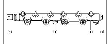
I. Rail. - 2. Fuel inlet from high pressure pump. - 3. Overpressure valve -4. Pressure sensor.
