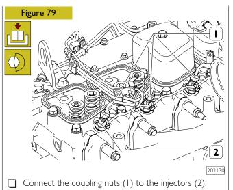
Tighten the fitting nuts (1).
