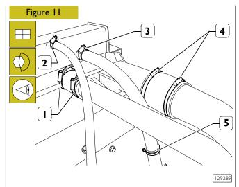
Connect the air and water pipes to the radiator assembly using the clamps (1, 2, 3 and 4) and the mounting bracket (5).
