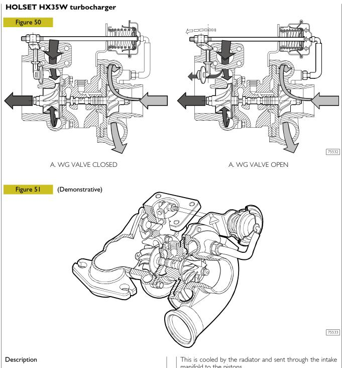
The turbocharger consists of the following main parts, a turbine, a valve for regulating the boost pressure, a central body and a compressor.
