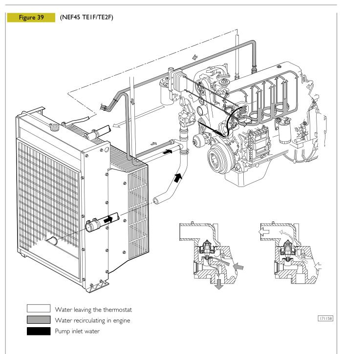
The heat exchange between the lubricant oil and the coolant (water), designed to keep the temperature within the established and control values, takes place inside of the heat exchanger. The coolant is sucked by a pump from the expansion tank, the position of which varies depending on the set-up of the engine; the fluid moves into the radiator through the conveyor and then into the flow regulator. The pump then sends the coolant to the heat exchanger (inside
