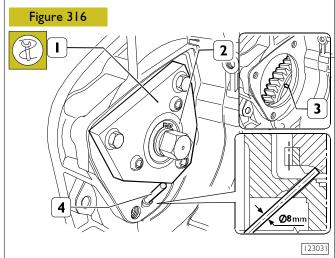
Fit tool 99360339 (1) to rotate the flywheel with the help of a wrench.
