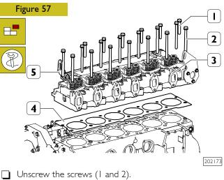
Using tool 99360595 via the lifting eyelets (5), remove the cylinder head (3) together with all the elements relating to the timing:
