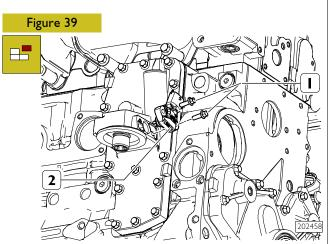
Unscrew the screws (1) and remove the oil pressure/temperature sensor (2).
