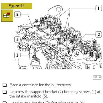
Unscrew the bracket (3) fastening screws (4).
