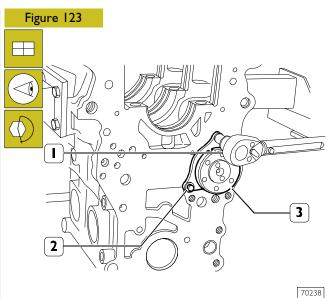
Place the plate (1) retaining the camshaft (3) with the slot facing the top side of the crankcase and the marking facing you, tighten the screws (2).
