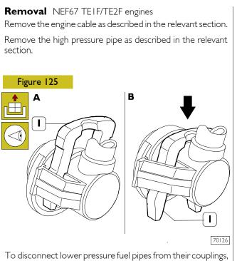
To disconnect lower pressure fuel pipes from their couplings, press clip (1) as shown in figure B.
