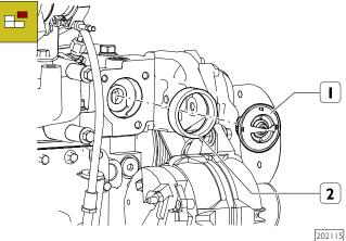
Remove the thermostat assembly (1).
