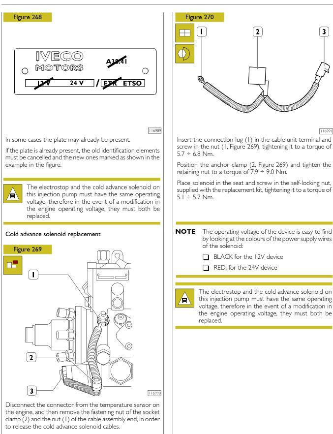
Remove the fastening nut (3) from the solenoid and remove the component from its seat.
