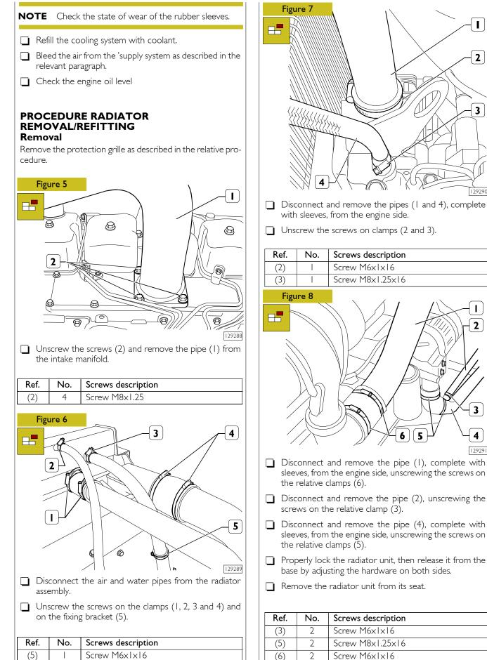
with sleeves, from the engine side. Unscrew the screws on clamps (2 and 3). Screws description Screw M6x1x16 Screw M8x1.25x16 2
