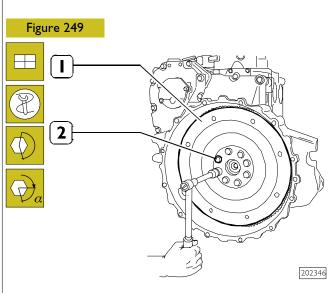
Tighten the screws (2) securing the engine flywheel (1).
