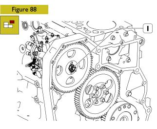
On the side of the timing gear, unscrew the nut (1) and recover the relative washer.
