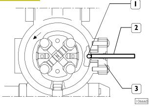
1. Slot on hydraulic rotor hub - 2. Synchronisation pin 99365196 - 3. Plate.
