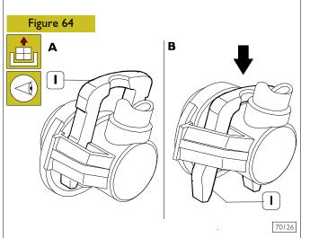
To disconnect lower pressure fuel pipes from their couplings, press clip (1) as shown in figure B.
