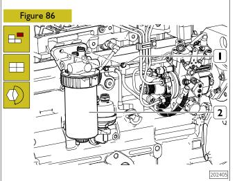
Unscrew the screws (1) securing to the crankcase.
