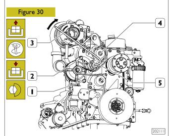
Unscrew the screw (1) anchoring the alternator to its lower support and the screw (2) securing the bracket.
